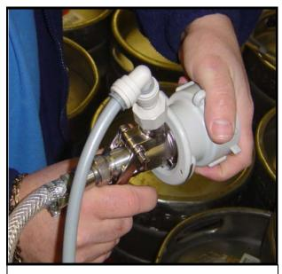
2) Fit the appropriate Empty Keg Simulator onto the coupler, and leave gas on
